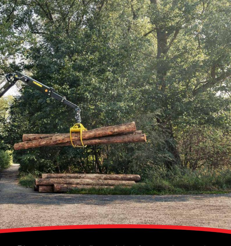
This cut-to-length timber handling crane is the perfect partner when your work consists of intense and heavy load cycles and where you from time to time need that extra capacity.
